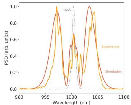
Fig 1. Spectral broadening with 26 bar Argon. Input: 1030 nm, 31 W, 10 MHz repetition rate.
