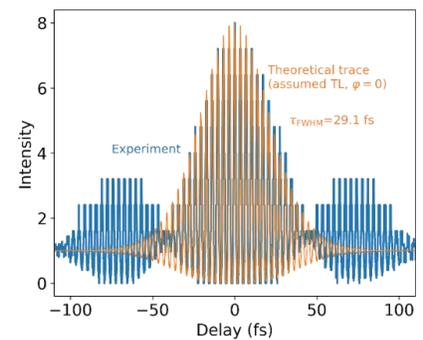
Fig 2. Interferometric autocorrelation trace of compressed pulse with SF11 prism compression.
